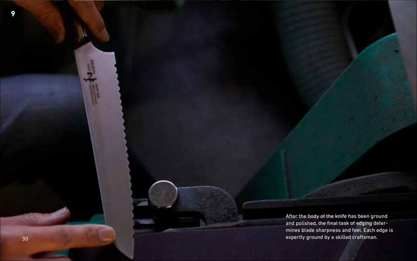
After the body of the knife has been ground and polished, the final task of edging determines blade sharpness and feel. Each edge is expertly ground by a skilled craftsman.
