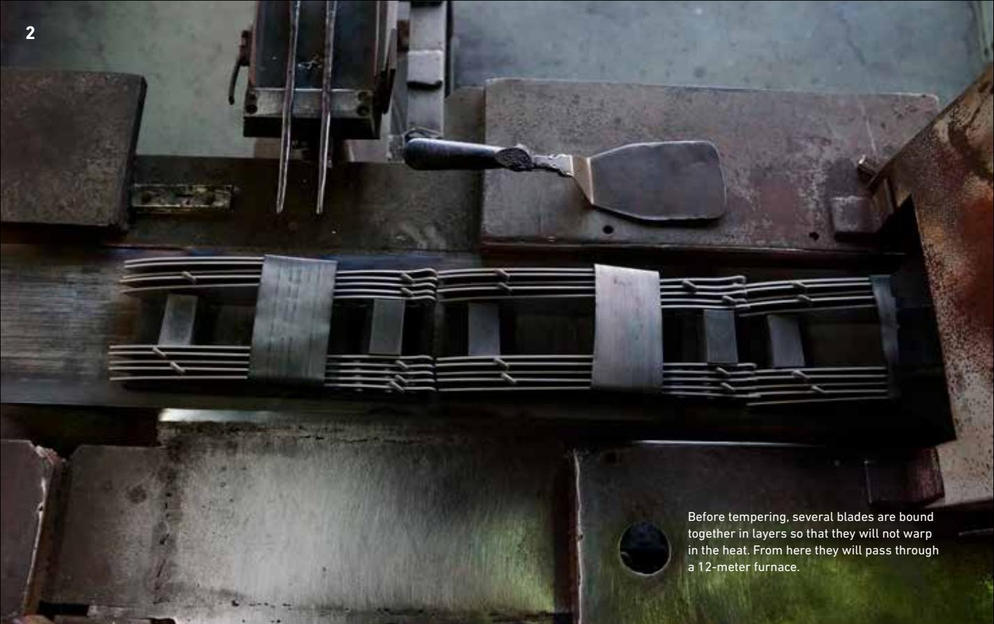
Before tempering, several blades are bound together in layers so that they will not warp in the heat. From here they will pass through a 12-meter furnace.
